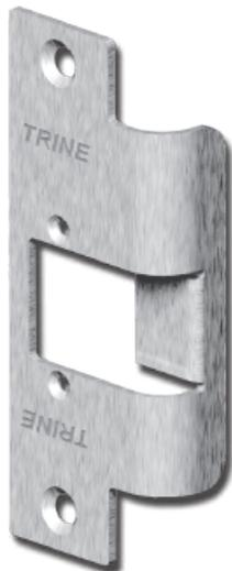
60% LESS FRAME CUTTING of Frame Face for ANSI 4 7/8" pre-prep frames. The strike opening on this face plate is offset by 3/16" the center to accommodate door sag for the 478 (just change faceplates, and use the same mechanism)
