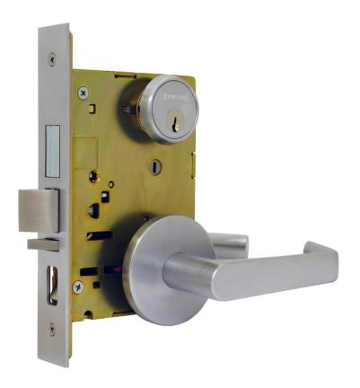
The SARGENT 8200 electrified mortise lock, is an ANSI/BHMA A156.13 Series 1000 Grade 1 mechanical mortise lock. It has a reversible stainless steel latch, independent non-handed stainless steel deadlatch.
