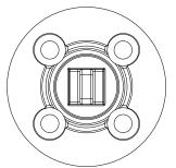
Make sure dummy spindle is aligned as shown
