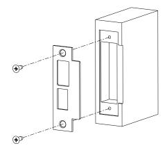
Step 3) Install spacer block on trim side of lock-body with 1/4" Fillister Head Screws
