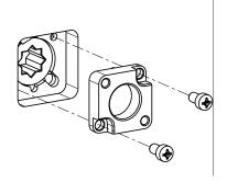
Step 4) Install adapter plate on trim side of door using 1/2" Flat Head Screws
