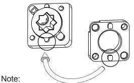
Align tabs on spacer with cutouts on lock-body
