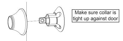
Step 4) Install lever on both sides of door with dowel screws
