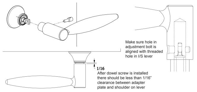
Step 8) Rotate both levers individually and make sure both levers return. If either lever binds, remove I/S lever and un-thread adjustment bolt 1/2 turn.
