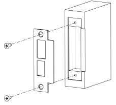
Step 2) Insert mortise lock into door and hand tighten longer 1" mounting screws
